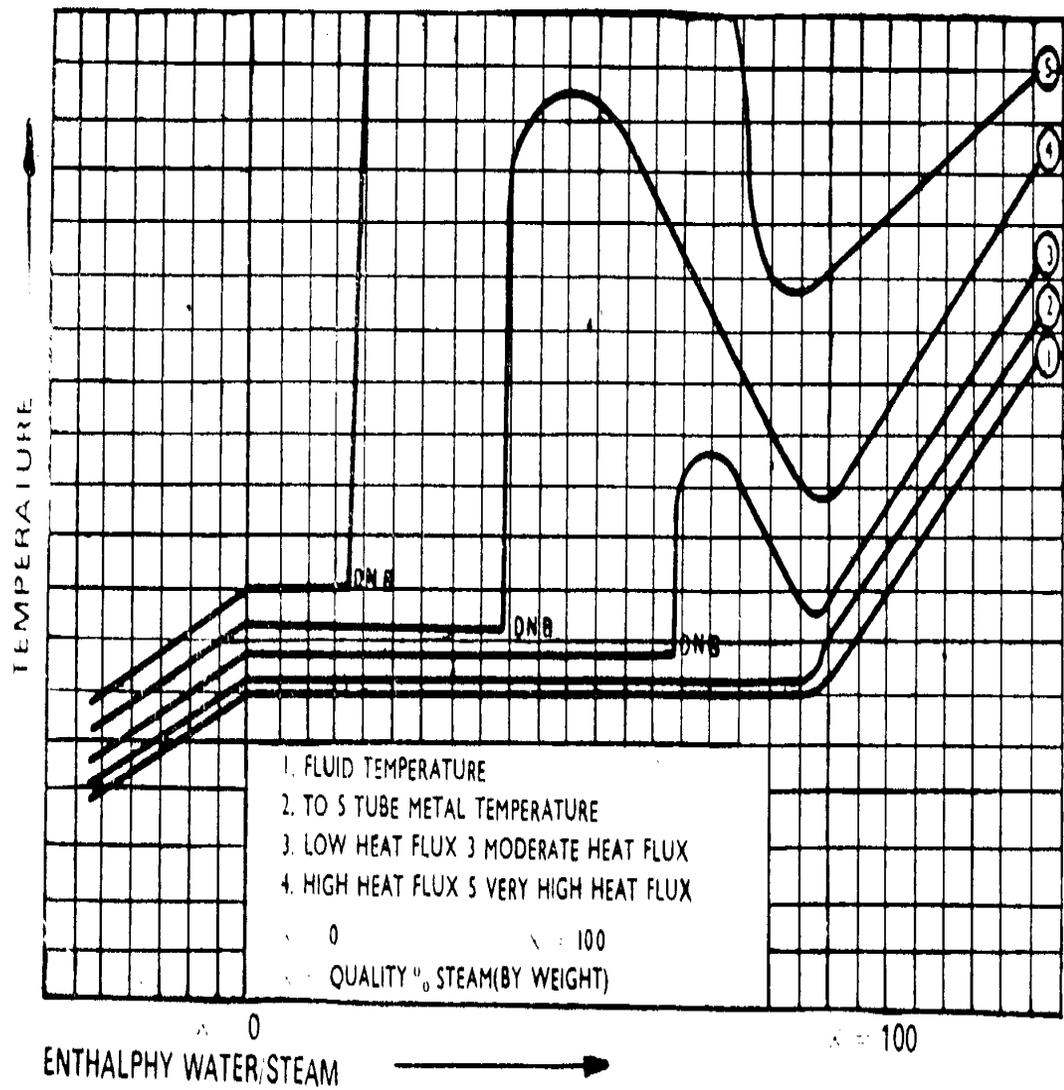
FIG.-3 OCCURRENCE OF DNB WITH DIFFERENCE OF HEAT FLUX
