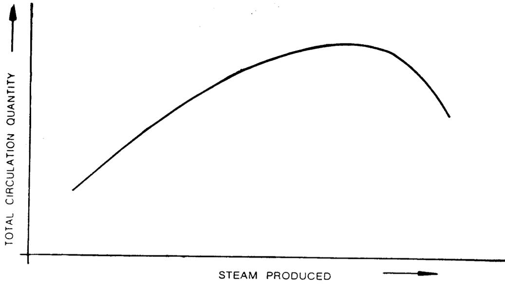
FIG. -4 CIRCULATION QUANTITY VS STEAM PRODUCED
