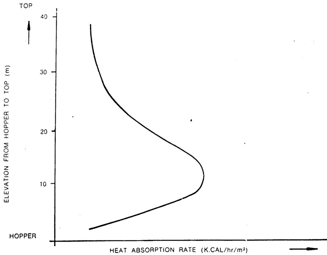
FIG.-5 HEAT ABSORPTION RATE ALONG THE RISER TUBES
