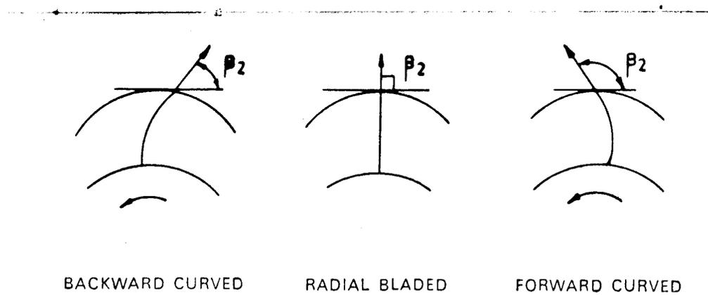
FIG. -1-CONFIGURATION OF BLADE
