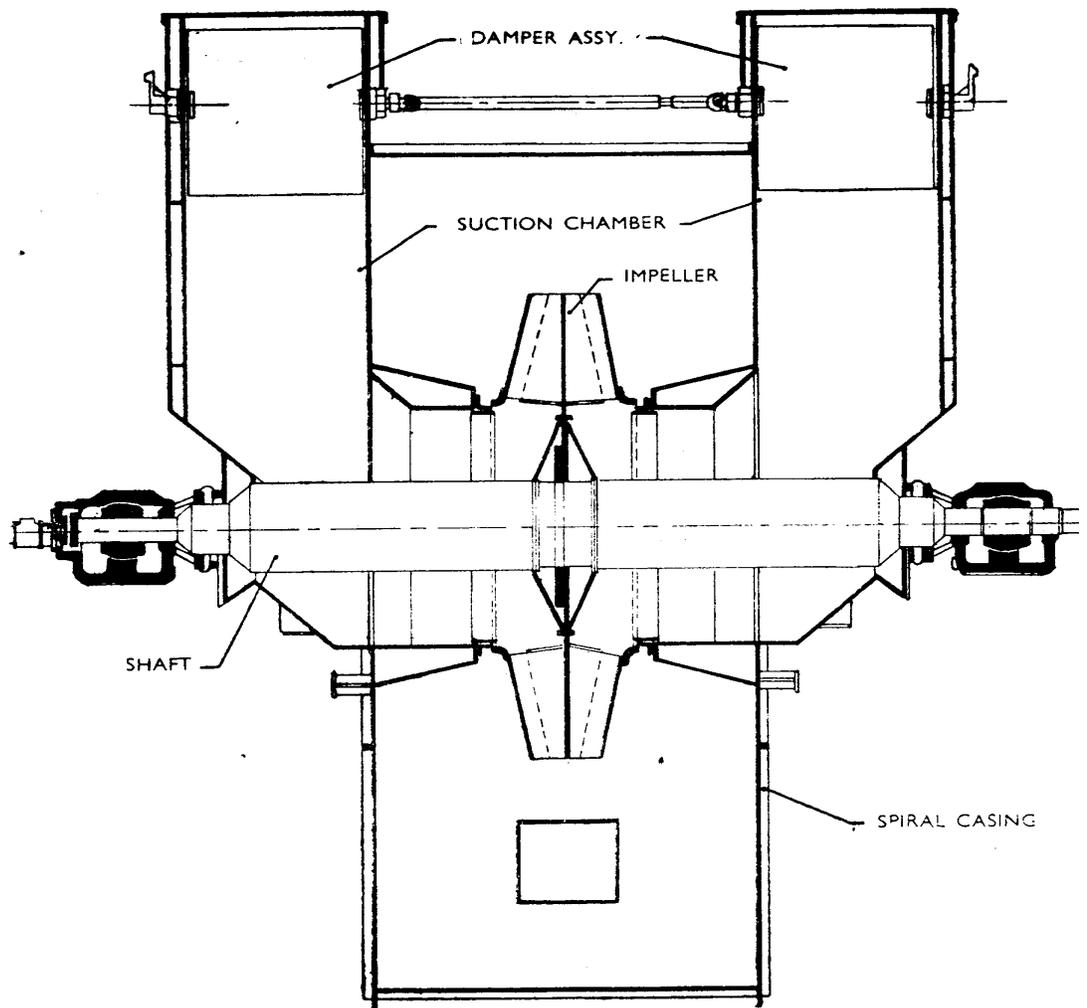
FIG. -5 DOUBLE SUCTION RADIAL FAN (NDZV)
