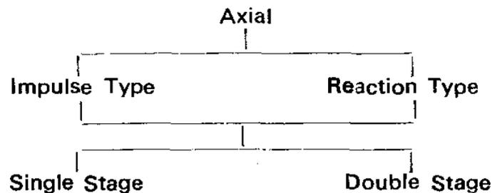
In axial flow fans the main flow is parallel to the axis of rotation of the fan both at entry and exit. Axial fans may be classified further into Impulse Type and Reaction Type fans.
