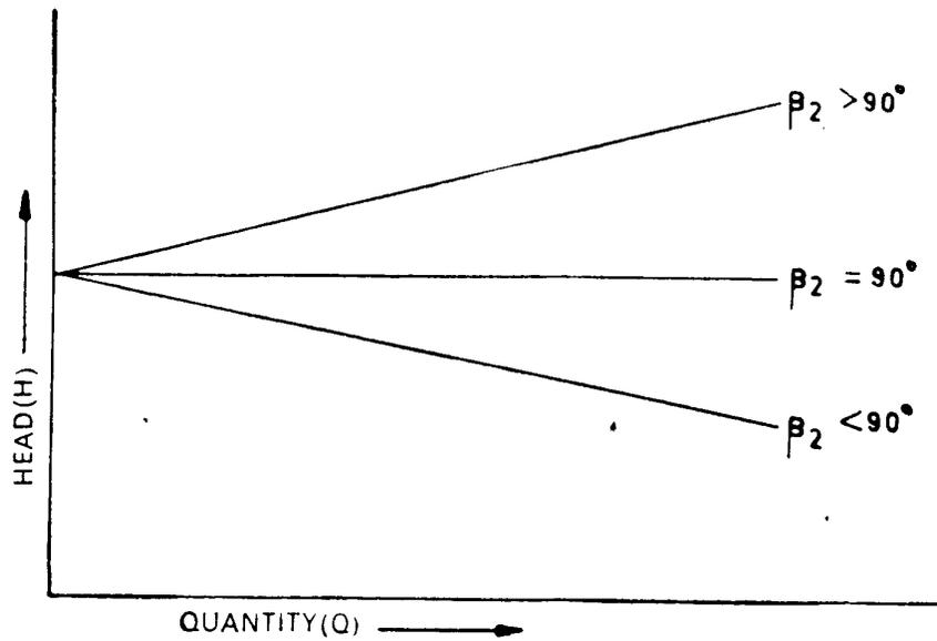
FIG. -2 CHARACTERISTICS OF RADIAL IMPELLERS
