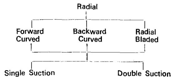
Based on the configuration of the blade with respect to the direction of rotation of the impeller (as shown in the Fig. -1 it is called Backward Curved, Forward Curved and Radial Bladed impeller. For better understanding it can be mentioned that the blade angle at exit X is less than 90° equal to 90° and greater than 90° in B.C. Bladed, Radial Bladed and F.C. Bladed Impellers respectively.
